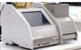
Infraneo Measurement of proteins, water content, starch, ash and other constituents Page 13
